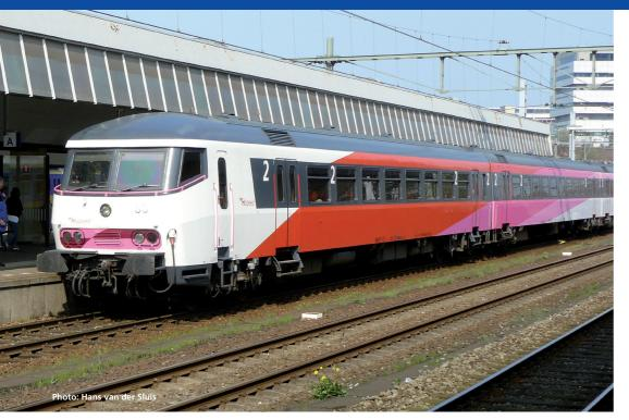
Known as Fyra, the Nederlandse Spoorwegen operated a rapid transit network in the Netherlands and Belgium. The operational capability of the AnsaldoBread multiple unit trains ordered for this purpose was delayed and subsequently remained inadequate, so that recourse was made to existing material in the form of partly modernized ICR car fleets. The sets operated as push-pull trains with class 186 locomotives and ICR control cars. In 2013, the Fyra brand was abandoned and replaced by NS Hispeed.
